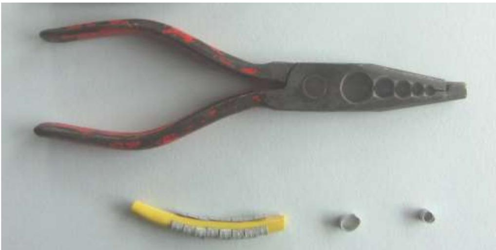
**Figure 6. Top: Pliers for closing Swift rings. Lower left: Swift rings as supplied by BTO. Lower right: Rings opened & closed.**
